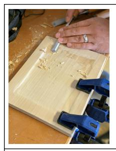
Using wood chiseling tools, carve out the inside rectangle to about  $\frac{1}{8}$  to  $\frac{1}{4}$  inch deep.
